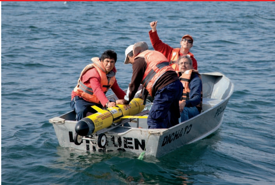
Researchers prepare to deploy an automated underwater glider to collect marine data.
